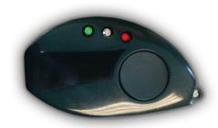
The hand-held tester is designed to operate autonomously in the field under any light conditions and to detect the presence of a taggant within a second, returning a YES or NO result.
